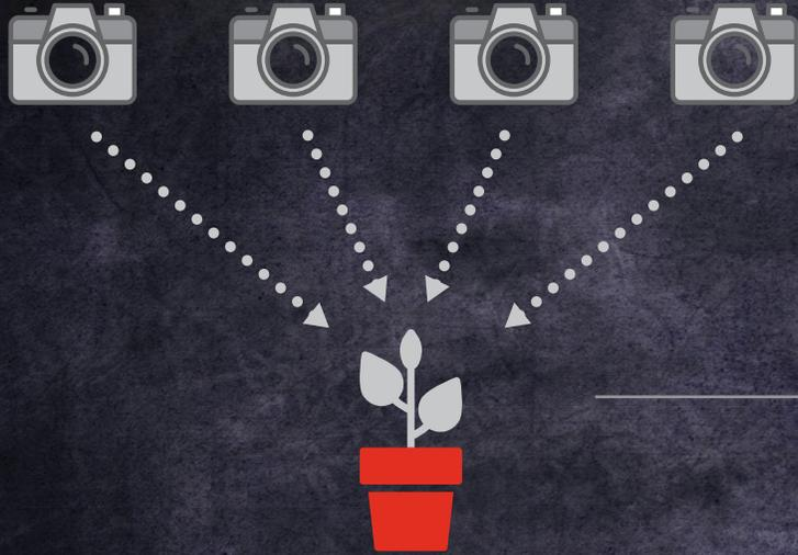
A system of multiple cameras arranged in order to capture multiple images of the same moment that can later be stitched together to create a spherical image.
